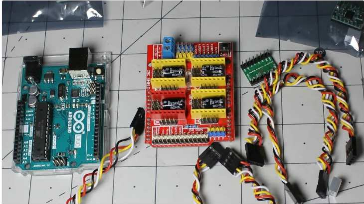
GRBL easily runs on an Arduino Uno (Source: Jeremy S Cook via Arrow)
